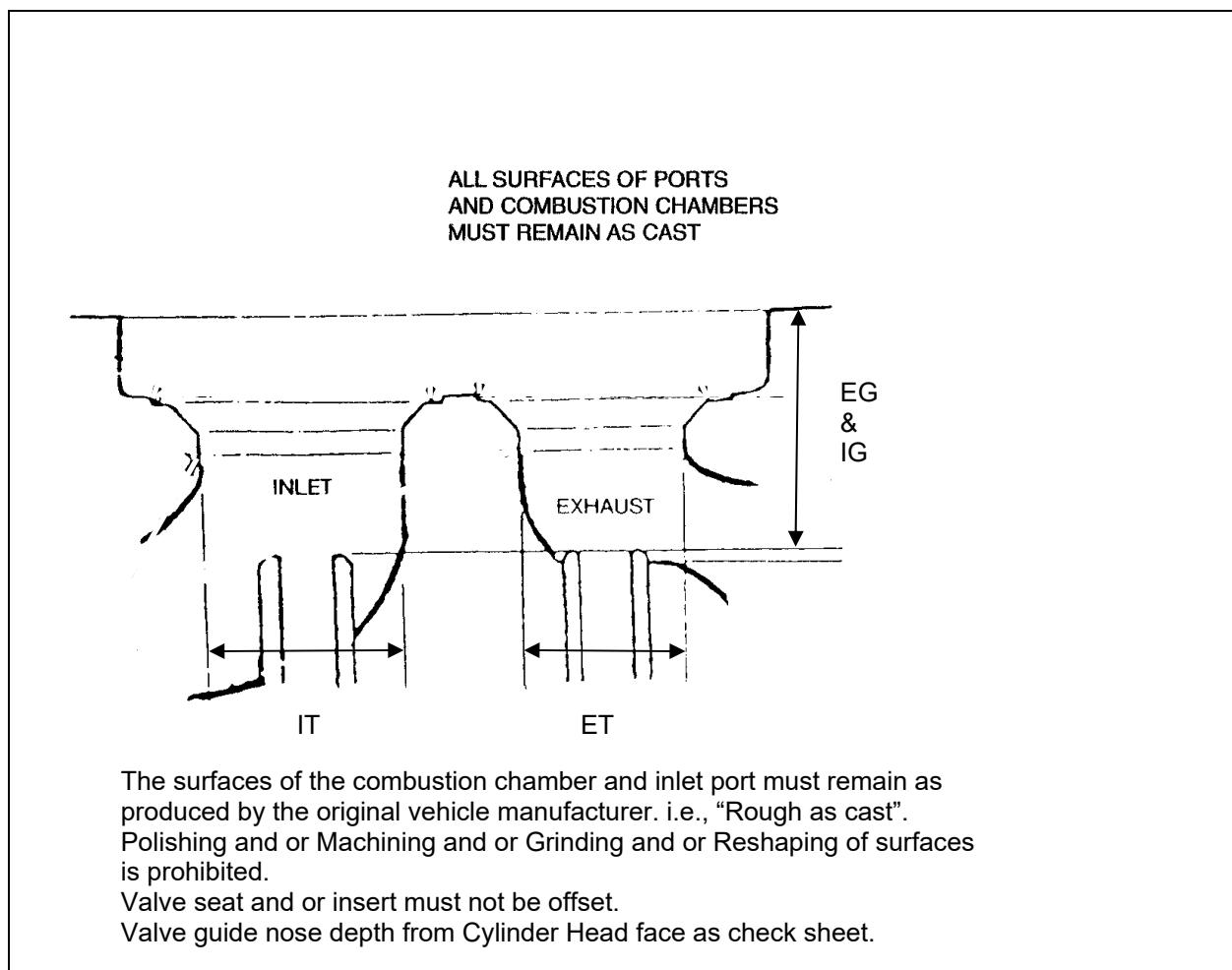
DRAWING No. 3 CYLINDER HEAD COMBUSTION CHAMBER.
