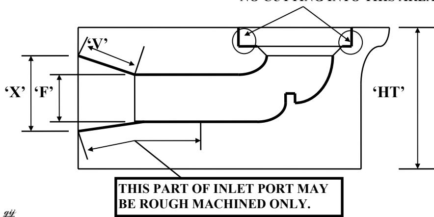
The surfaces of the inlet and exhaust ports must remain as produced by the original vehicle manufacturer. i.e., "Rough as cast". Polishing and or Machining and or Grinding and or Reshaping of surfaces other than shown is prohibited. "3 Angle cut" to valve and valve seat permitted. Reshaping and or cutting into the combustion chamber base adjacent to a valve insert as part of the "3 Angle Cut" process is prohibited.
