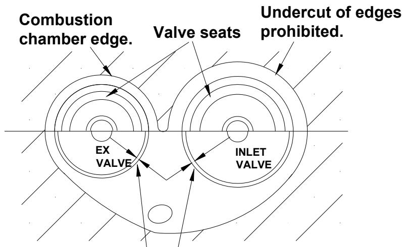
**Valve to Valve seat edge distance
