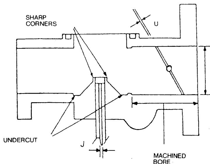
DRAWING No. 2 CYLINDER HEAD INLET &amp; EXHAUST PORTS.
