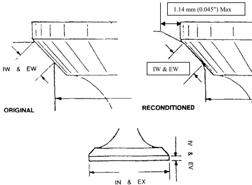
Valve Insert top face must be below or In Line with Combustion Chamber Face.
